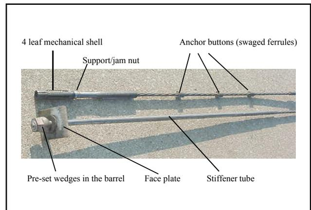
Figure 3 – A tensionable cable bolt (Design 1)
