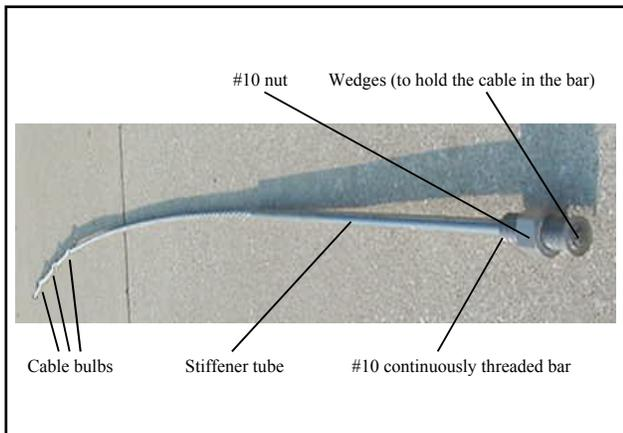
Figure 4 – A tensionable cable bolt (Design 2)
