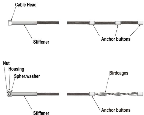
Figure 2: Typical cable bolt components
